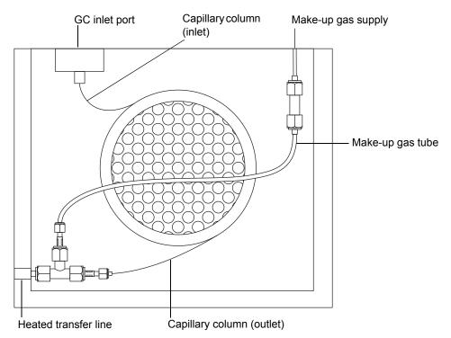
A make-up gas is supplied coaxially to the capillary column via a T-piece connected to the heated transfer line. An auxiliary EPC unit installed on the Agilent GC supplies and controls the make-up gas. To maintain constant make-up gas flow as the oven temperature changes, the make-up gas tube is configured as an auxiliary GC column that operates in constant-flow mode. The length of the make-up gas tube within the oven is critical, and only a Waters engineer should install it.
