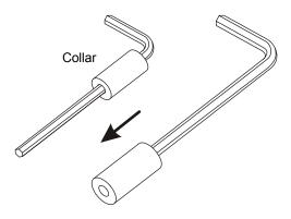
6. Insert the collar into the sample cone.
