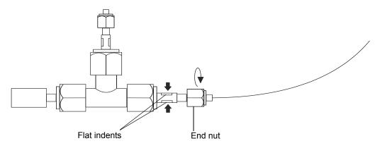
B Installing the GC Column
