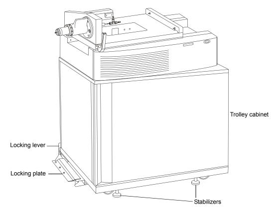
The APGC trolley is a mobile steel cabinet on top of which the APGC is fixed in place. A locking lever and locking plate engage or disengage the trolley and mass spectrometer.
