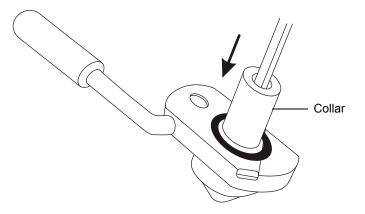
**Notice:** To avoid damaging the fragile sample cone, do not place it on its tip; instead, place it on its flanged base.
