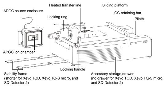
When you operate the mass spectrometer in GCMS mode, the APGC source enclosure and APGC ion chamber serve in place of the standard mass-spectrometer source enclosure and cone gas nozzle.
