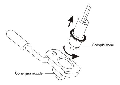
8. Remove the sample cone from the tool.
