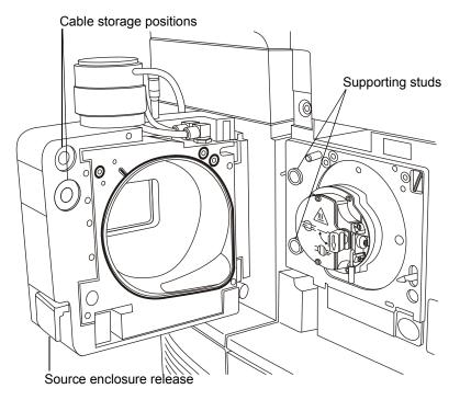
8. Store the cables neatly by plugging them into the cable storage positions on the rear of the source enclosure.
