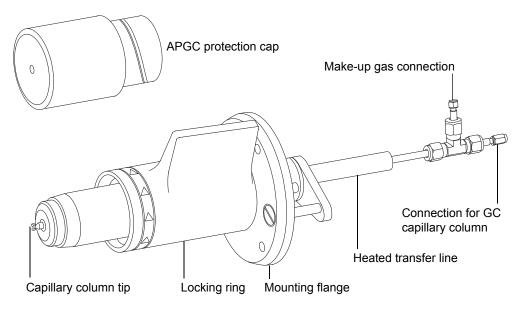
The heated transfer line positions the capillary column tip in the correct location relative to the APGC ion chamber within the mass spectrometer's source enclosure.
